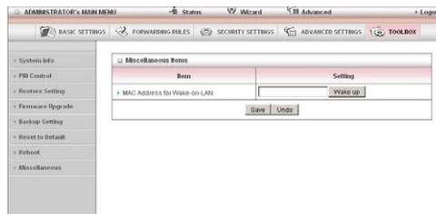
Wake-on-LAN enables the router to start-up a computer or device (if the computer supports it) when a WOL packet is detected on the network going to the client MAC you have entered.
