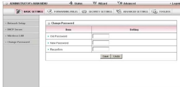
This page allows you to change the 3G25W-R web configuration password. Please type in the old password (the factory default password is admin) and then type in the new password. Type the same new password in the “Reconfirm field” and click “Save”.
