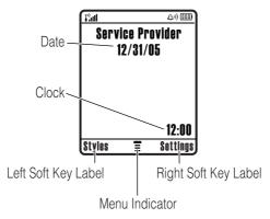
The Menu Indicator shows that you can press to open the menu. Soft Key Labels show the current soft key functions. For soft key locations, see page 1.
