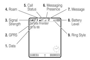
1. Data Indicator – Show connection and data transmission status. The Bluetooth® wireless connection indicator ≱ shows when a Bluetooth connection is active. Other indicators can include:
