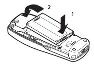
**3** Align the cover over the back of the phone, placing the end of the cover approximately 1/4 inch past the end of the phone. Lower the back cover onto the phone.
