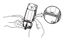
**5** Once the battery is released from the latch, it will lift slightly so that it can be removed from the phone.
