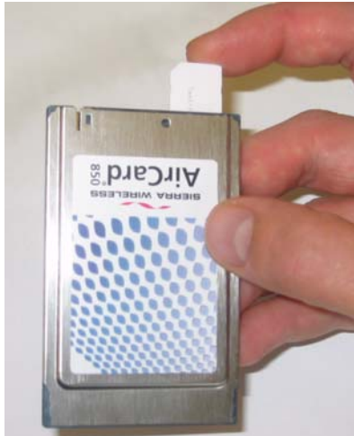
Figure 2-1: Inserting the SIM card into the AirCard modem SIM card slot
