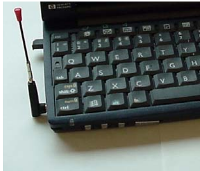
Figure 5-1: Proper positioning of the AirCard modem antenna
